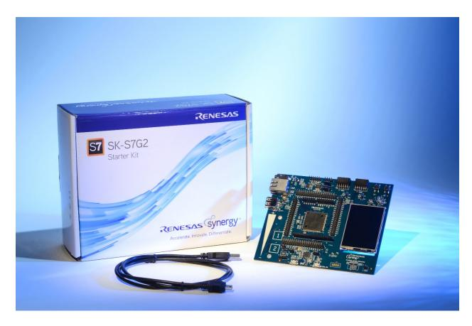
All Renesas Synergy starter kits come with an industry standard high speed Segger J-Link OB debugger as well as an integrated Bluetooth<sup>®</sup> low energy (BLE) module. The Bluetooth chipset used on the SK-S7G2 is based on the Renesas RL78/G1D.
